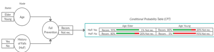
Figure 1. Illustrative example of a BN, where the conditional probability distribution function of a node labeled “Fall Prevention” is represented by a Conditional Probability Table (CPT). The CPT of this node incorporates the states of its parent nodes “Age” and “History of Falls”.
